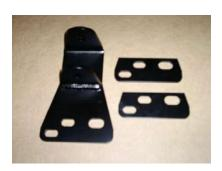
BETWEEN BRACKET AND CROSS MEMBER(the spacers used are determined by the amount the body overhangs the rear crossmember which is unique to individual vehicles, it maybe necessary to use the 2mm spacer 4mm spacer or both for the bracket to be level with the body) USING THE 3 M10 BOLTS NUTS & WASHERS SUPPLIED.
